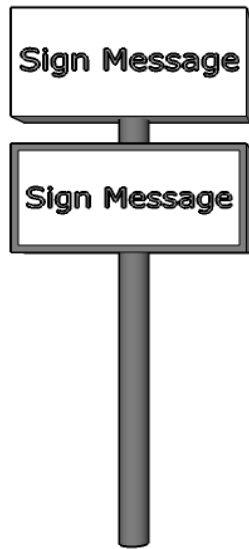
Figure 7.3 : Multi-faced signs (A) that can be viewed from more than one (1) direction should be flush (back-to-back) (B).
