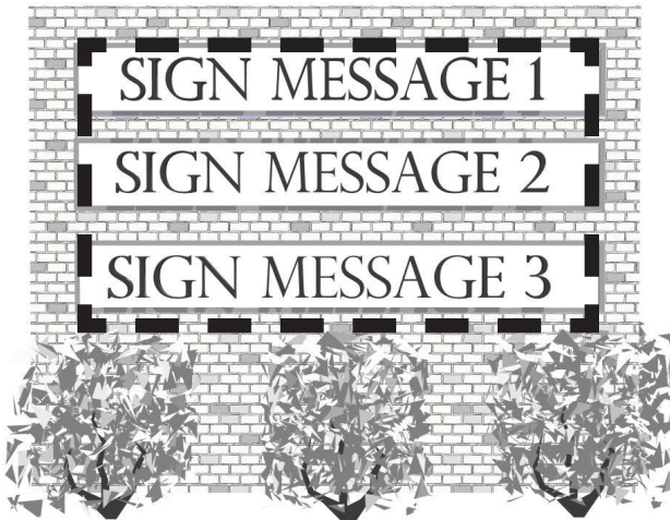
Figure 7.5 :Space between signs is calculated as part of sign face for signs with multiple faces (A)(B).
