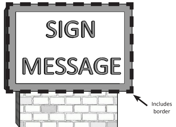
Figure 7.2: Sign Area also includes any material or color forming an integral part of the display or used to differentiate the sign from the backdrop
