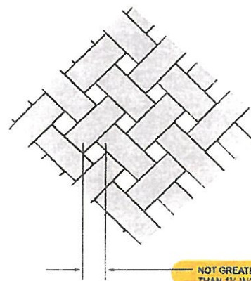
Commentary Figure 305.2.8 MAXIMUM OPENING WIDTH IN BARRIERS BUILT WITH DIAGONAL MEMBERS
